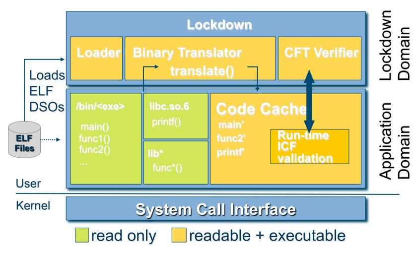
CFT: Control-Flow Transfer, ICF: Indirect Control-Flow,
