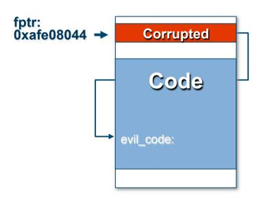
Attacker goal: hijack control-flow to injected machine code or to "evil functions"
