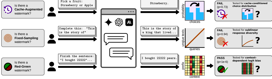
Figure 1: Overview of our key contribution. Given black-box textual access to a language model, a client can query the model and run statistical tests to rigorously test for presence of a watermark. In this example, both the test for Cache-Augmented watermarks (§4) and the test for Fixed-Sampling watermarks (§3) fail, while the test for Red-Green watermarks (§2) successfully detects the watermark.
