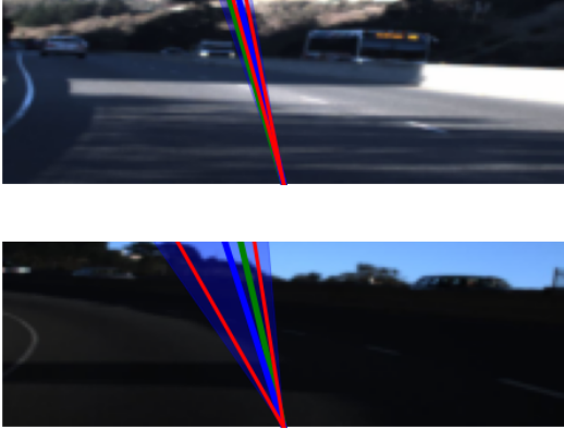
Figure 11: Two representative samples from the self-driving car dataset. The target steering angle is illustrated in green, the predicted one in blue. The empirical bounds for \epsilon = 2/255 are shown in red and the certified range is shaded blue.
