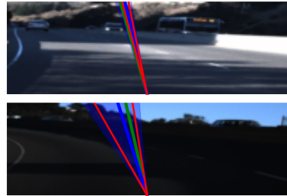
Fig. 15. Samples from the self-driving car dataset. The target steering angle is illustrated in green, the predicted one in blue. The empirical bounds for \epsilon = 2/255 are shown in red and the certified range is shaded blue.
