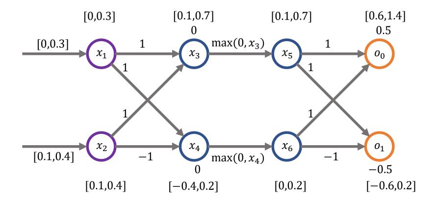
Using Box, we succeed in proving the network classifies any input in the range as 0. This is because **[0.6,1.4] > [-0.6, 0.2]**, provably so.
