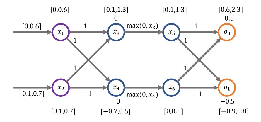
Using Box, we failed to prove the network classifies any input in the range as 0, even though property actually holds. This is because **[0.6,2.3] is not > [-0.9, 0.8]**, provably so.
